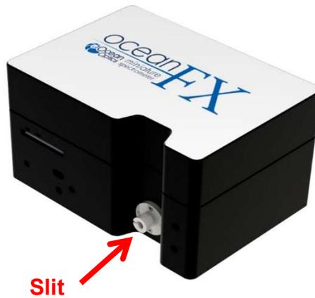
2. Use the Allen key to remove the 2 the screws attaching the slit to the spectrometer.
