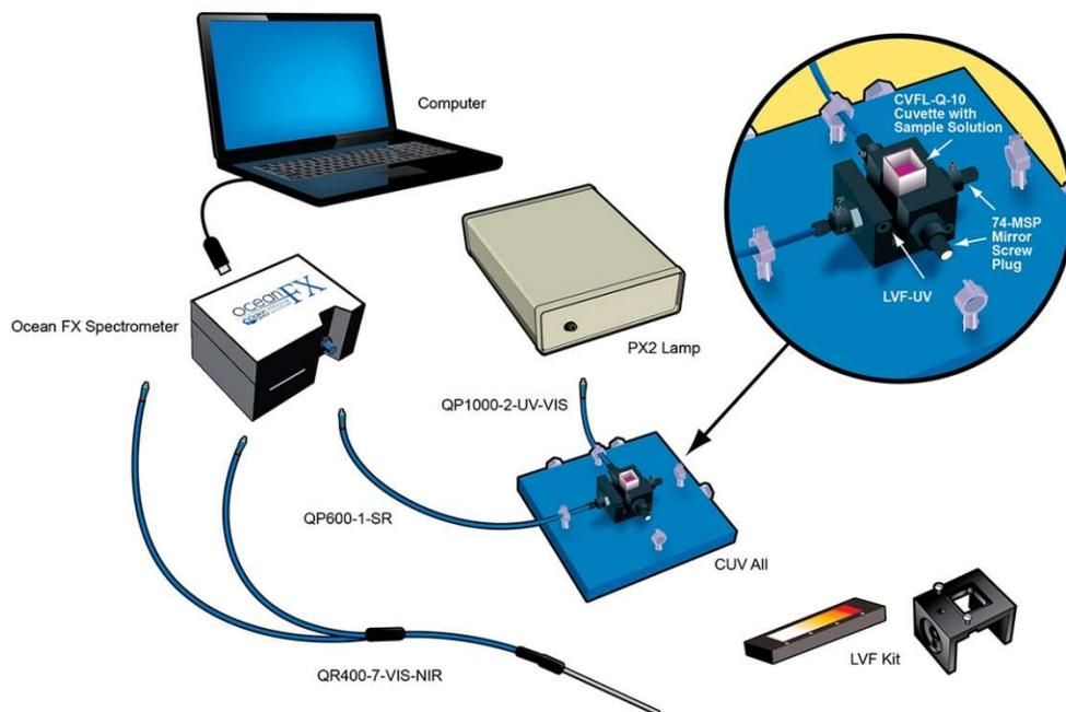
Typical Fluorescence Set Up with an LED Excitation Source at  $90^\circ$
