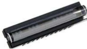
8. **Detector:** Ocean FX utilizes a Hamamatsu S11639-01 linear silicon CMOS array detector. Similar to CCD detectors, a CMOS detector also converts incident photons into an electric charge. But each CMOS detector pixel has an amplifier attached that transfers the accumulated charge after a measurement has been made to the A/D converter. CMOS detectors can typically operate at much higher speeds than CCD detectors.
