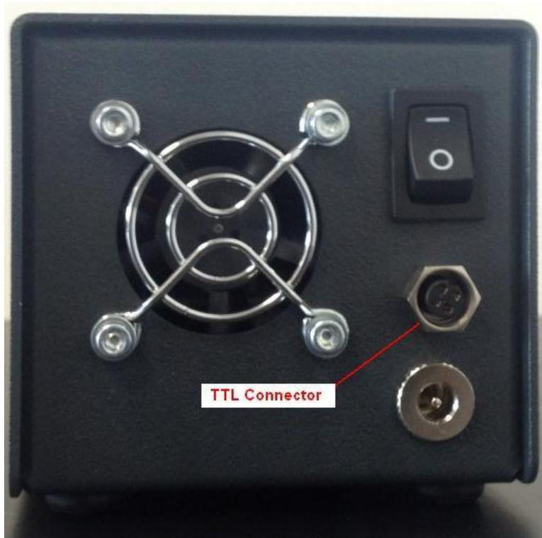
The pinout of the TTL connector is as follows:
