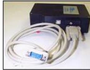
**HR2000 Spectrometer with the USB-ADP-PX2 and the PX-2 DB15 Cable**
