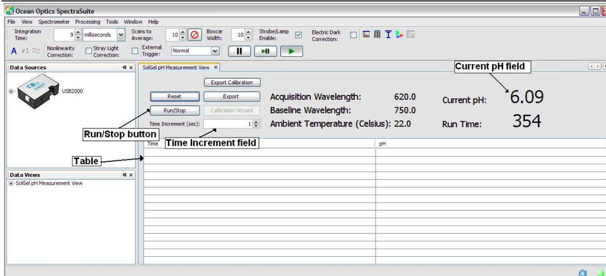
2. Click the **Run/Stop** button to toggle data acquisition appearing in the lower table on the screen. Data is recorded at the time interval you specify in the **Time Increment (sec)** field.
