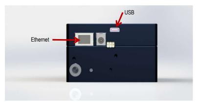
**Rear View of Ocean FX Spectrometer**
